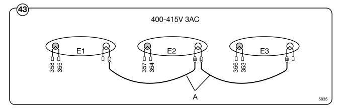
• Take off wire L3 (A) from terminal L3 on isolator Q1 and from terminal 6 on heating relay K21.
